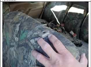
Step 3. Driver and Passenger Tops/DT & PT: Tuck the fabric under the plastic for the headrests. Then tip the backrest forward, slide the seat ahead, and tuck the hook Velcro™ into the seat.
