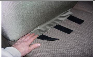
**Step 5. Driver & Passenger Top/DT&PT**: Slide the seat covers on with the long hook (fuzzy)  $Velcro^{TM}$  to the front.
