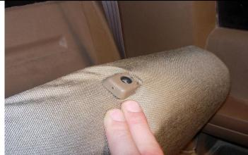
**Step 6. Driver & Passenger Top/DT&PT**: Tuck the seat covers under the plastic for the headrests. Next, tuck the long hook Velcro<sup>™</sup> into the seat and mate them to the loop Velcro<sup>™</sup> sewn inside the back edge.
