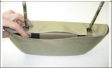
Step 7. Headrests/H: Slide the covers on with the long hook straps to the front. Mate them to the loop  $Velcro^{TM}$  sewn inside the back edge.
