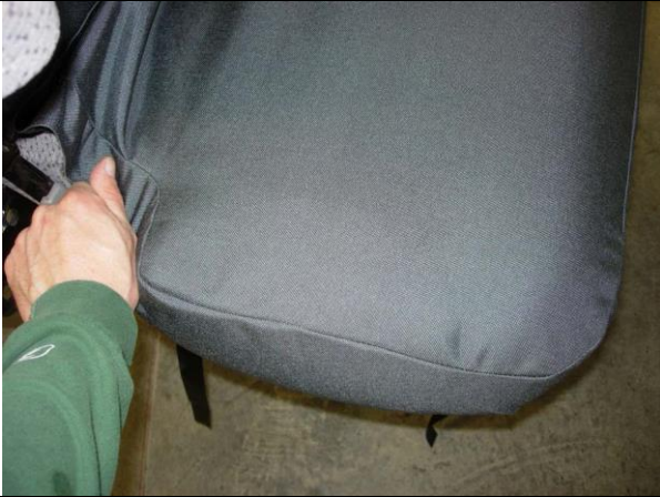
Step 15. Bottom/B: Pull the cover around the back left and right corners.
