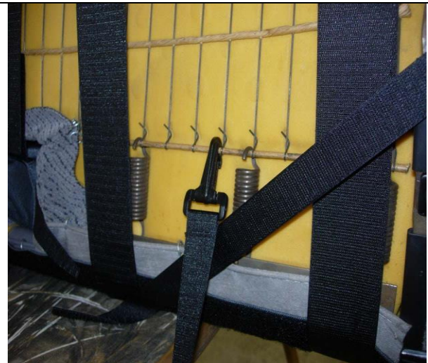
Step 22. Bottom/B: Clip the three plastic Velcro™ buckles where shown, over the metal bar, then press it onto the rear loop Velcro™ on the left, middle and right passenger areas.
