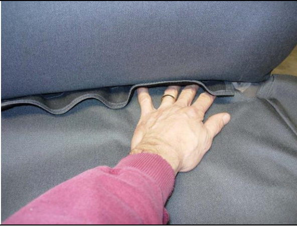
Step 7. Driver and Passenger Bottoms/DB&PB: Tuck in the back edge of the seat cover.
