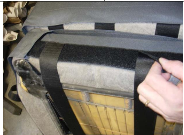
Step 10. Driver and Passenger Bottoms/DB&PB: Route the long hook Velcro™ under the seat and connect it to the loop Velcro™ sewn on the back edge.
