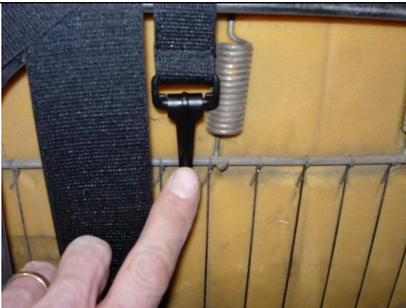
Step 11. Driver and Passenger Bottoms/DB&PB: View from under the back of the seat bottom. Snap the two plastic buckle over the small metal bar, keeping them about 6-8" apart. This will help keep the seat cover in place.
