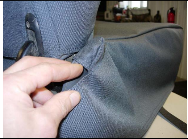
Step 8. Driver and Passenger Bottoms/DB&PB: Pull the outside part of the seat cover over the small piece of the seat as shown, line up the hole in the cover for the recline lever and put the lever back on.
