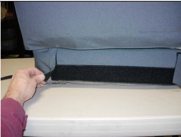
Step 9. Driver and Passenger Bottoms/DB&PB: Pull the sides of the seat cover around to the back and connect the Velcro™ as shown.
