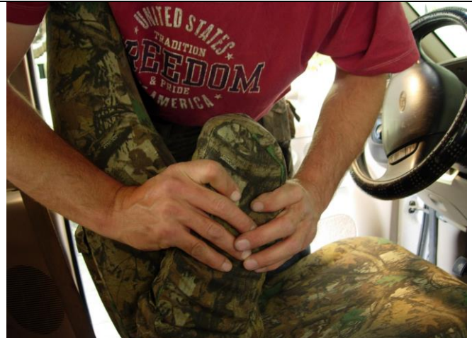
Step 14. Driver and Passenger Armrests/DA&PA: Work the armrest cover on all the way using both hands from top to bottom.
