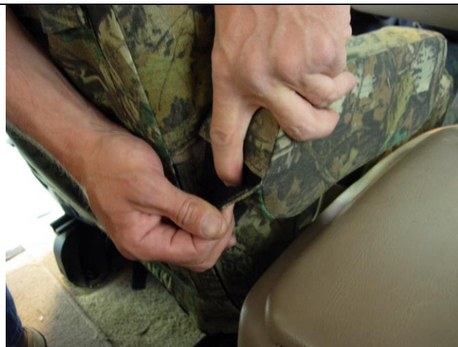
Step 15. Driver and Passenger Armrests/DA&PA: Mate the fasteners at the back of the armrest covers as shown.
