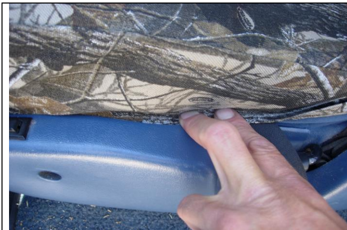
Step 19. Driver & Passenger Bottoms/DB&PB: Tuck the fabric of the seat cover behind the plastic on the outside edge of the seat.
