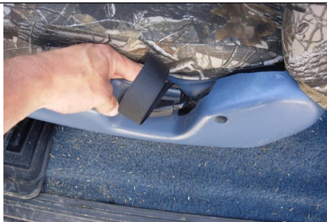
Step 20. Driver & Passenger Bottoms/DB&PB: Tuck the Velcro™ behind the recline lever and angle it to the back.
