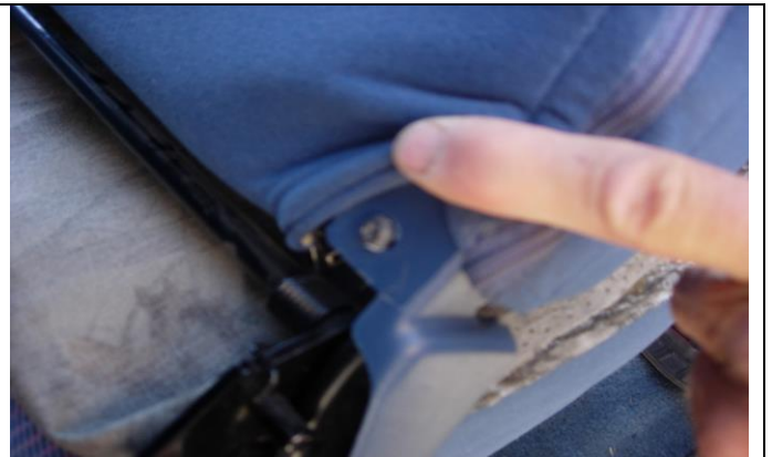
Step 2. Bottom: Tip the seat forward, lift the upholstery and remove this screw.
