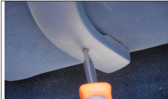
Step 1. Bottom/B: Remove this screw from the plastic on both sides.
