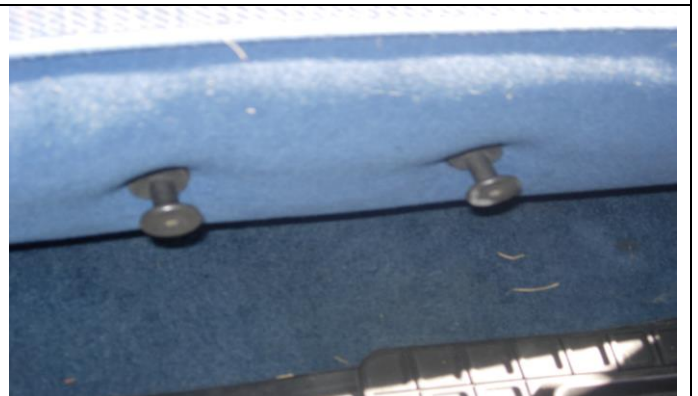
Step 4. Bottom: Temporarily remove the plastic cup holders if it has them, by lifting up. Use a # 25 Torx bit to temporarily remove the bolts. Once the bottom cover is installed, cut a small X where each hole is, and then put the bolts back in.
