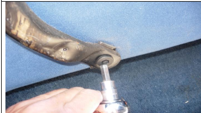
Step 3. Bottom: Remove this 5/16" stud bolt on both sides. Wipe off any grease or dirt on the metal arms after removing it from the bottom.
