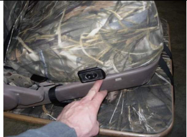
Step 10. Driver & Passenger Bottoms/DB&PB: Place the cover on, positioning it by the lumbar cut-out. Partly tuck in the back edge of the cover and line up the seams as in Step 2.
