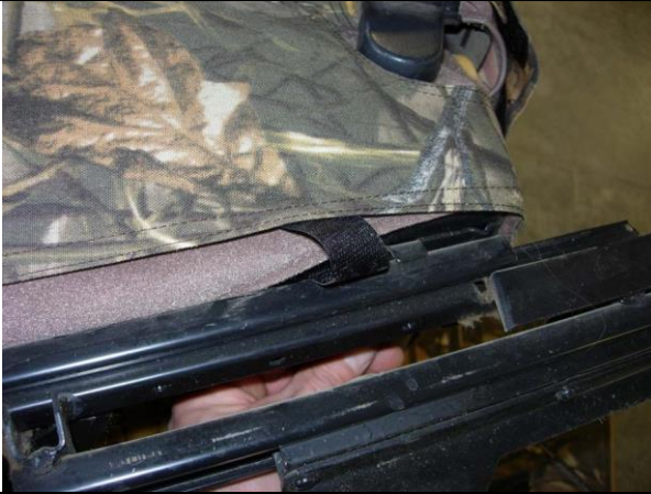
Step 11. Driver & Passenger Bottoms/DB&PB: Route the inside Velcro™ over the seat slide.
