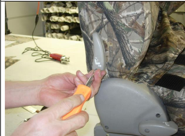
Step 21. Driver & Passenger Top/DT&PT: Re-install the levers.
