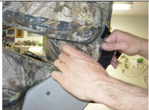
Step 22. Driver & Passenger Top/DT&PT: Carefully pull the fabric under the armrest.
