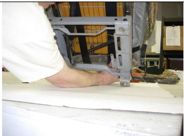
Step 12. Driver & Passenger Bottoms/DB&PB: Route the front edge Velcro™ avoiding the seat mechanisms as shown..
