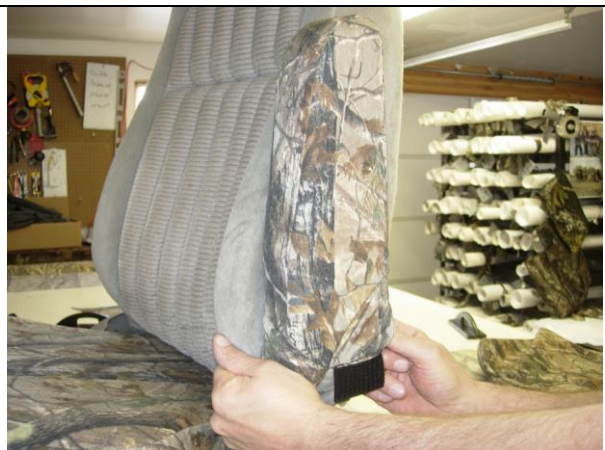
Step 30. Driver & Passenger Armrests/DA&PA: Keep pulling the cover down. It will be very tight.
