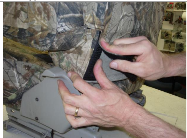
Step 24. Driver & Passenger Top/DT&PT: Connect the vertical Velcro™ starting on top.
