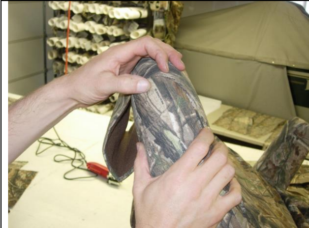
Step 19. Driver & Passenger Top/DT&PT: Continue working the seam fabric inward on top.
