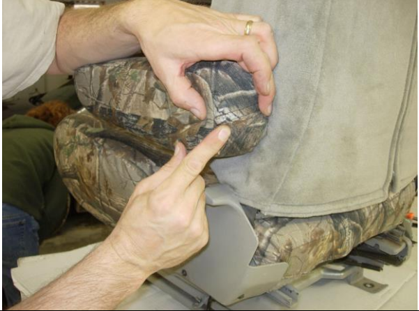
Step 34. Driver & Passenger Armrests/DA&PA: Keep working at it until you get the fabric meeting at the back.
