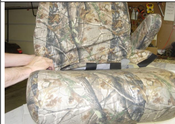
Step 17. Driver & Passenger Top/DT&PT: Work each side down equally when pulling it down
