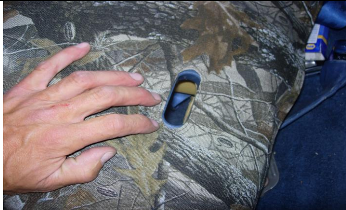
Step 7. Bottom: Center the cut out for the seat belts.
