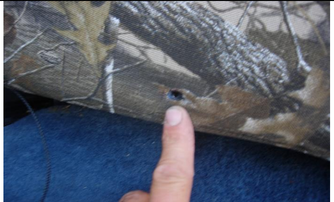
Step 8. Bottom: Pull the sides of the seat cover back and line up the hole for the backrest bolt.
