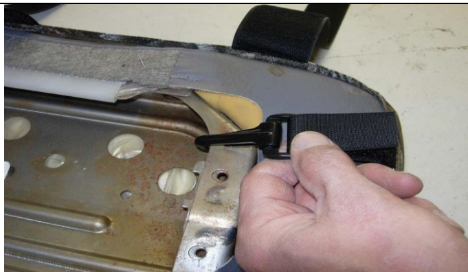
Step 11. Bottom: Clip the plastic side buckles over the metal edge of the seat or a seat support wire. Note, this is not a picture of the actual seat. The 1992-98 installation was updated to accommodate the new buckles.
