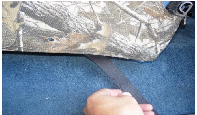
Step 10. Bottom: Route the long outside edge hook Velcro™ at an angle, over the top of the seat slide to the loop Velcro™ sewn on the back edge of the seat cover. Lastly, tighten and re-connect the hook Velcro™ to the loop Velcro™ sewn on the back edge of the seat cover, lining up the openings for the seat belts and side bolts.
