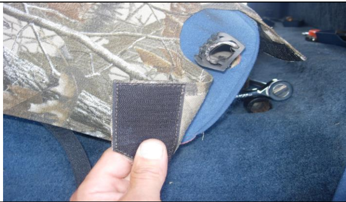
Step 9. Bottom: Pull the side around to the back and press it to the loop Velcro™ sewn on the back edge of the seat cover.
