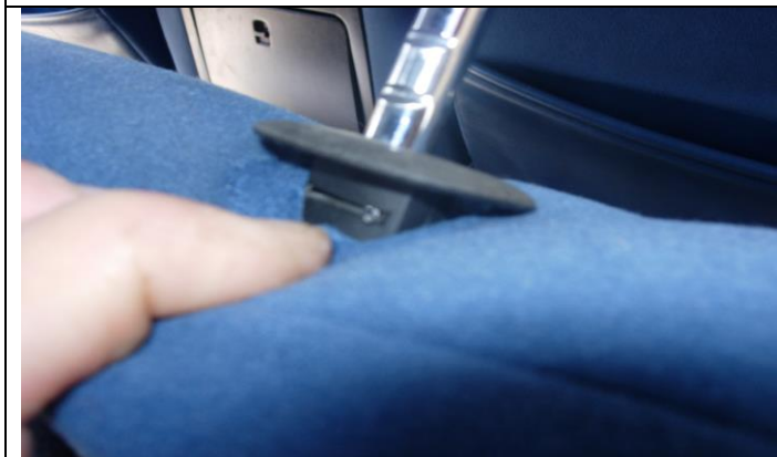
Step 5. Top: Temporarily remove the headrests by pushing the material down to expose this clip. Lift the headrests up all the way and keep gentle upward pressure while pulling back on both clips until you feel them release. Don't try to remove the clips.
