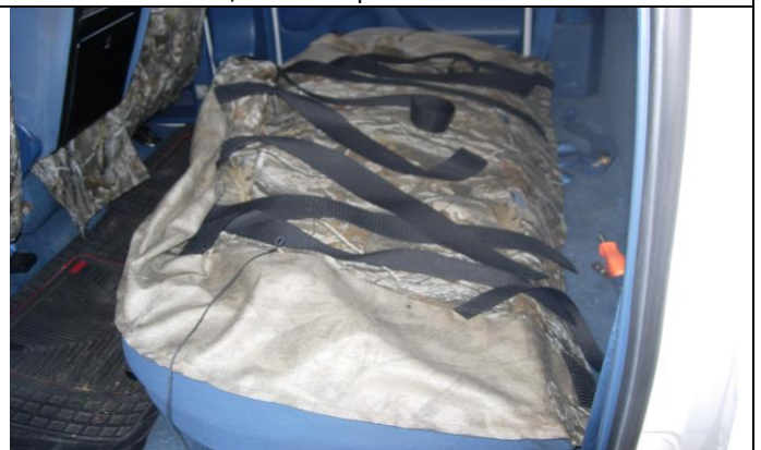
Step 6. Bottom: Place the seat cover on with the long hook (sticky) Velcro™ to the front as shown.
