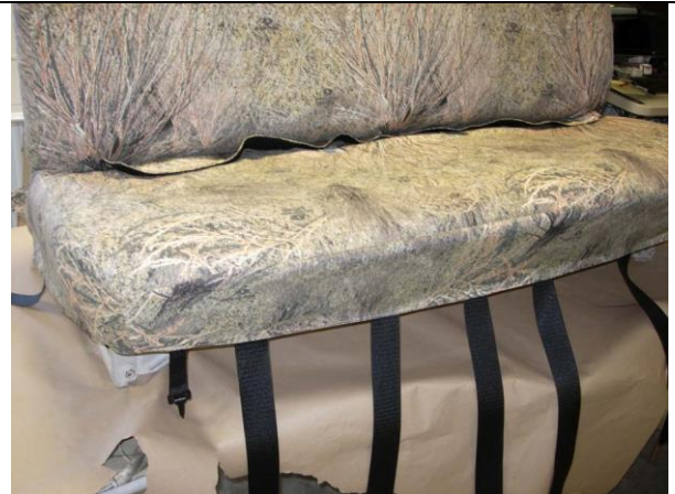
Step 8. Bottom/B: Carefully disconnect the Velcro™ on the seat cover, and place seat cover on with the long hook Velcro™ to the front. Same as Step 4, line up the seams of the seat cover to the seams of the seat, they should closely match.
