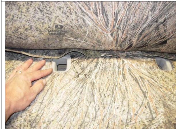
Step 9. Bottom/B: Tuck the back edge into the seat.
