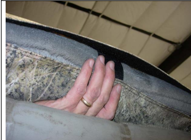
Step 7. Top/T: Using one hand in a smoothing action down the front of the seat from the top to the bottom, tighten the front of the seat cover. Use the same hand to pin the hook (sticky) Velcro™ to the seat, then press the loop (fuzzy) Velcro™ to it.
