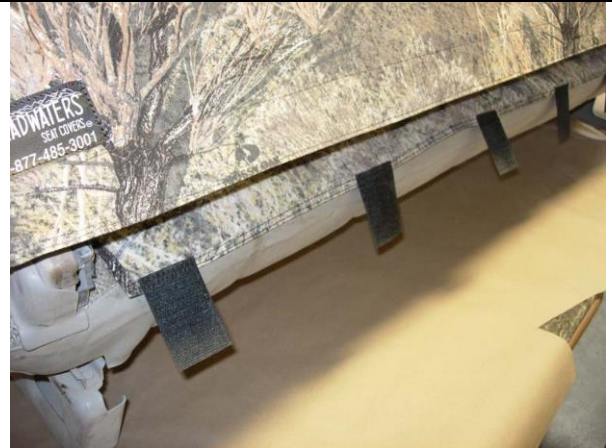
Step 6. Top/T: Pull all the Velcro™ thru to the back.
