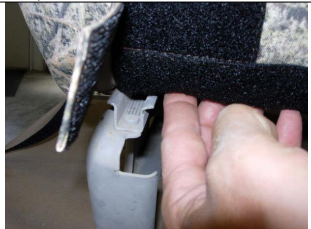
Step 10. Bottom/B: Tuck the back loop Velcro™ on top of the seat slide as shown.
