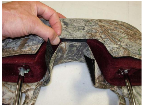
Step 22. Headrests/H: Fasten the center Velcro™ first.
