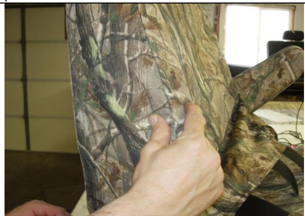
Step 18. Driver & Passenger Top/DT&PT: Same as Step 2 & 9, center the cover by lining up the seams on left and right. Work the seam fabric inside the cover from thumb to forefinger, or towards the main body.
