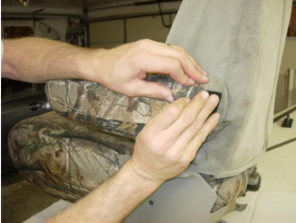
Step 31. Driver & Passenger Armrests/DA&PA: Work the front inside of the armrest around the corner and fold the armrest down. This will be the toughest. Push the cover over the top of the armrest.
