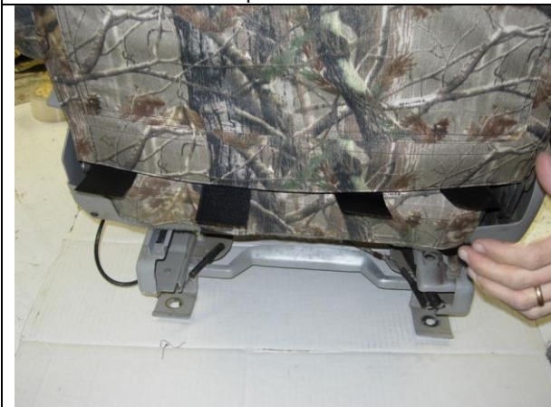
Step 27. Driver & Passenger Top/DT&PT: Carefully pull the fasteners one by one to the back.
