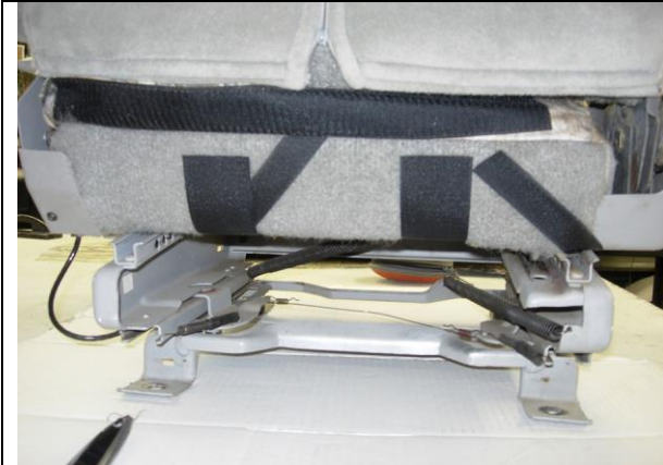
Step 13. Driver & Passenger Bottoms/DB&PB: Route the outside edge Velcro™ at roughly a 45 degree angle and press them to the carpet on the seat.
