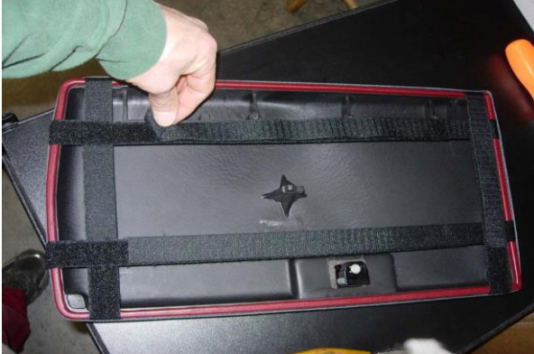
Step 34. Lid/L: Place the lid cover on with the top cut-out to the driver's side. Connect the Velcro™ under the lid. Keep re-tightening the Velcro™ for the best fit.
