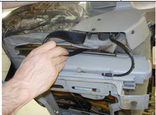
Step 10. Driver & Passenger Bottoms/DB&PB: Route the inside edge hook (sticky) Velcro™ over the seat slide where shown.
