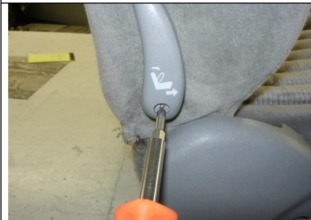
Step 15. Driver & Passenger Top/DT&PT: Temporarily remove the access lever using a Phillips screw driver.
