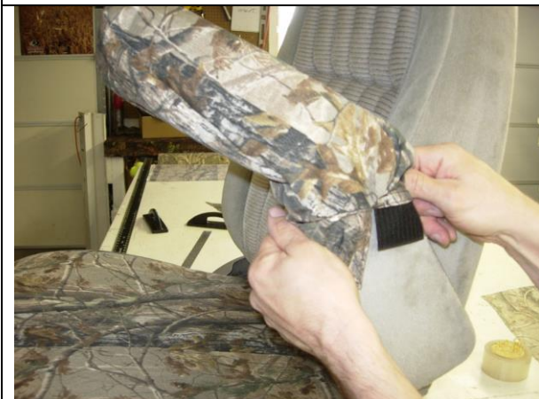
Step 29. Driver & Passenger Armrests/DA&PA: With the armrest up, carefully slide the cover on.
