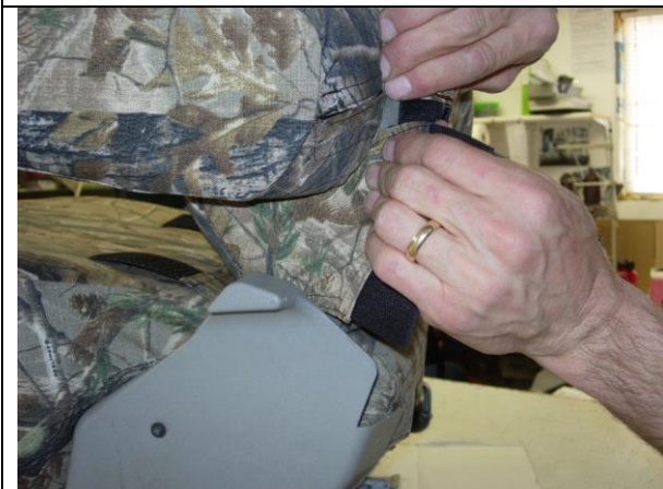
Step. 23 Driver & Passenger Top/DT&PT: Connect the small Velcro™ behind the armrests.
