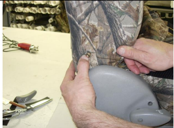
Step 20. Driver & Passenger Top/DT&PT: Line up the hole for the access lever. Note: Suburban, Yukon, and Tahoe do not have these entry levers
