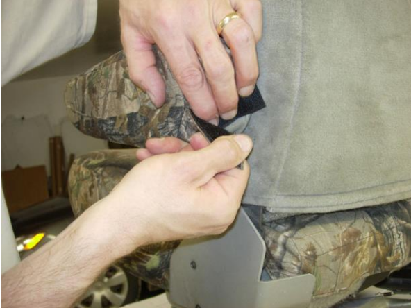
Step 33. Driver & Passenger Armrests/DA&PA: Tuck the hook Velcro™ in by covering it with the top hand while pressing the loop Velcro™ to it.
