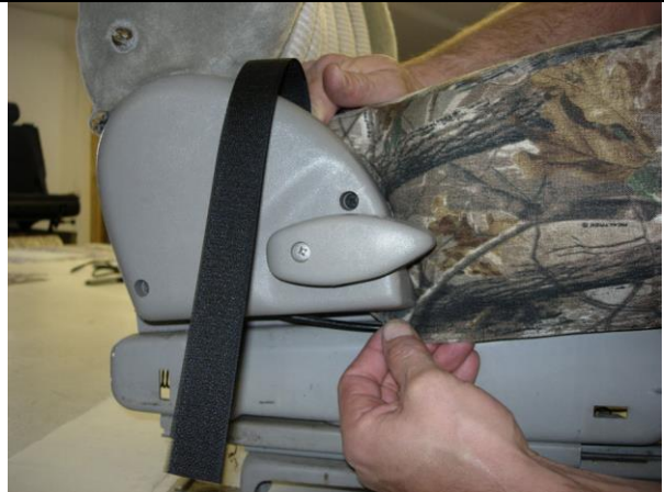
Step 8. Driver & Passenger Bottoms/DB&PB: Then, work the fabric into the front of the plastic.
