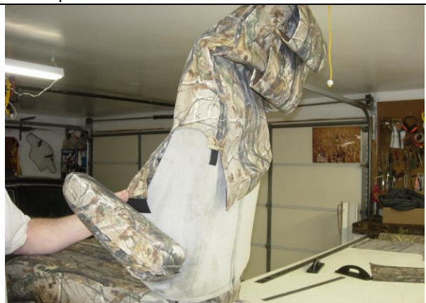
Step 16. Driver & Passenger Top/DT&PT: Carefully open the seat cover and pull it down into position.
