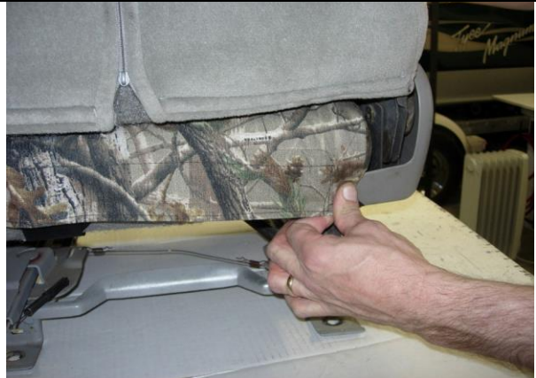
Step 14. Driver & Passenger Bottoms/DB&PB: Pull the back edge of the seat cover over both back corners and pull the cover back, press the Velcro™ to the carpet on the seat.
