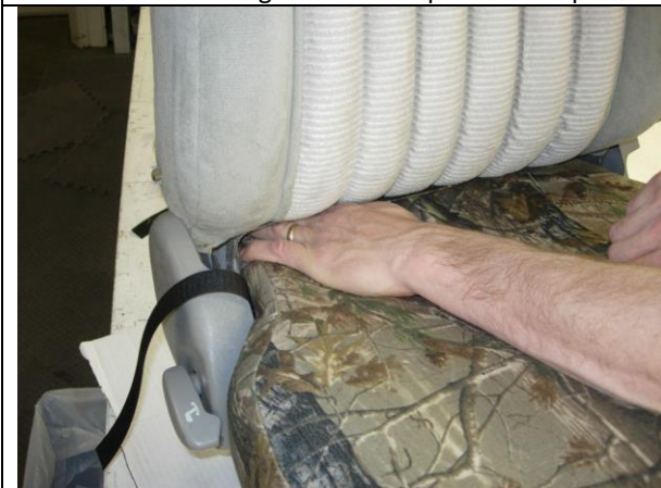
Step 9. Driver & Passenger Bottoms/DB&PB: Tuck the outside back edge in, but don't fasten it yet. Again, as in Step 2, line up the seams of the seat cover to the seams of the seat on left and right.
