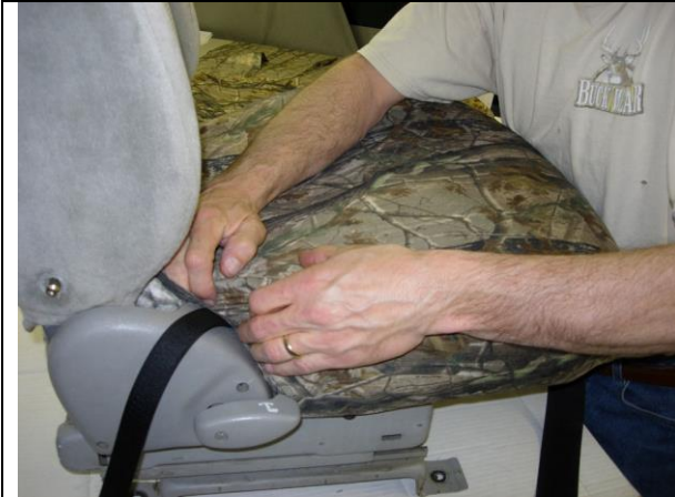
Step 7. Driver & Passenger Bottoms/DB&PB: Work the outside edge behind the plastic on top.
