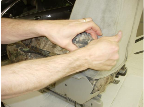
Step 32. Driver & Passenger Armrests/DA&PA: Use one hand to compress the armrest (left hand), and use the other hand to pull it around the back corner.
