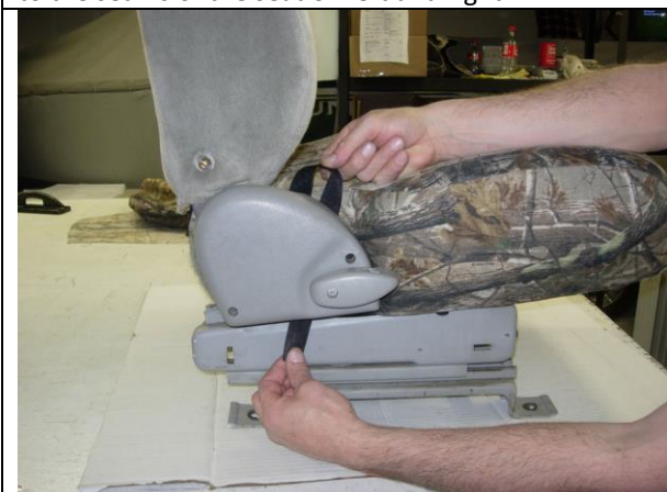
Step 11. Driver & Passenger Bottoms/DB&PB: Route the outside edge Velcro™ where shown.
