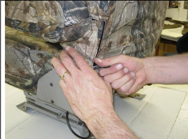
Step 25. Driver & Passenger Top/DT&PT: Re-connect for to line up material flush for best fit.
