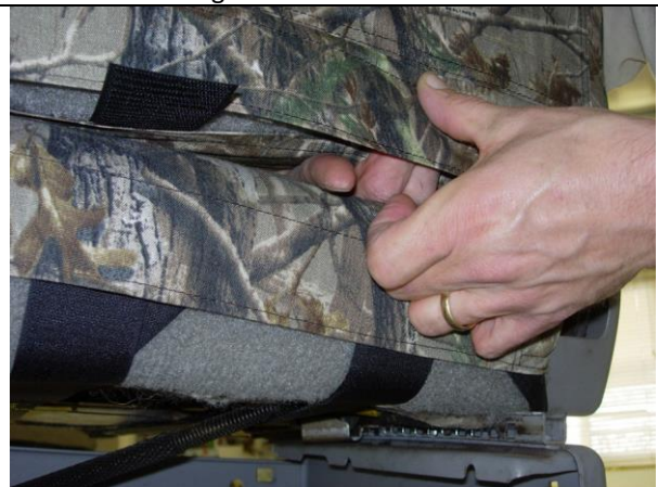
Step 28. Driver & Passenger Top/DT&PT: Pull on the Velcro™ from behind with one hand while using the other hand in a smoothing action down the front of the seat from top to bottom. Then pin the fastener to the seat with the front hand, and press the seat cover in. Work from one side to the other.
