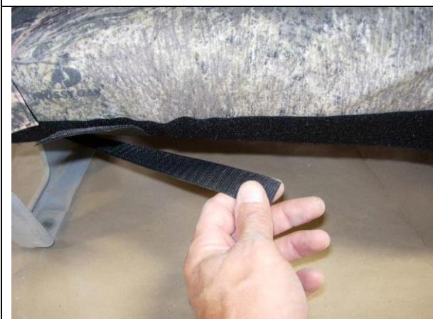
Step 15. Bottom/B: Again, route the side Velcro™ after the seat is in its normal position.
