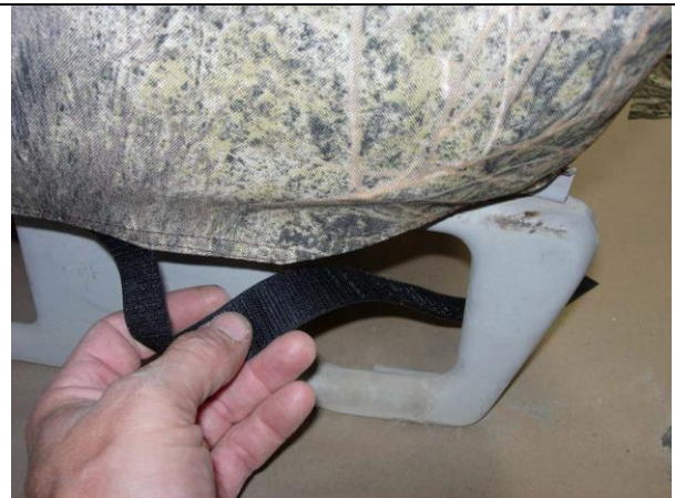
Step 14. Bottom/B: Route this side Velcro™ thru the rectangle opening in the framework after the seat is in its normal place. If connected beforehand, the Velcro™ can be damaged or torn when the seat is slid back into position.
