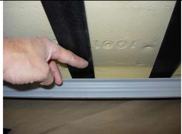
Step 12. Bottom/B: Route the long front hook Velcro™ over the top of the metal bar under the front of the seat as shown.
