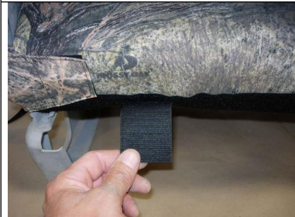
Step 13. Bottom/B: Connect them to the loop Velcro™ sewn on the back edge as shown. Tighten the seat cover similar to Step 7, using one hand in a smoothing action from front to back, take up the slack and connect the Velcro™.
