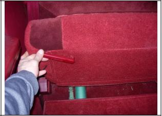
**Step 4. Bottom/B:** Pull the lever under the passenger side and lift the seat bottom partway up.
