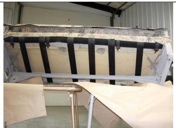
Step 10. Bottom/B: Connect the front Velcro™ to the back edge as shown. Also shown are the anti-slip buckles. See Step 11 for close up on the connection.
