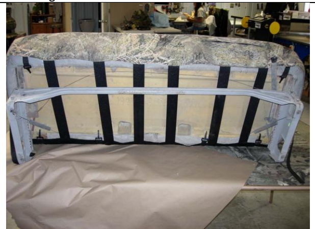
Step 8. Bottom/B: Route the front hook Velcro™ above the grey metal bar and seat slide wire as shown.
