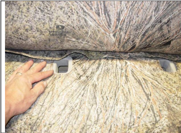
Step 5. Bottom/B: Tuck the back edge in, lining up the seat belt openings.
