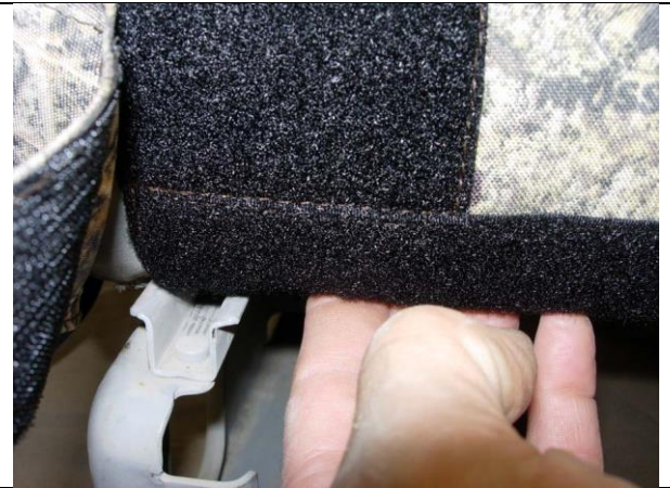
Step 6. Bottom/B: View from behind the driver side bottom. Pull the back edge down as shown.
