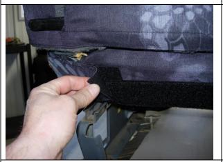
**Step 13. Bottom/B:**Pull the left and right side around to the back and connect the Velcro™
