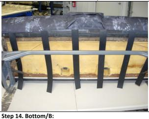
Line up the seams of the seat cover to the seams of the seat. Route the front hook Velcro™ above the grey metal bar and seat slide wire as shown.
