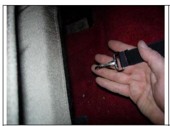
Step 5. Driver & Passenger Bottom/DB&PB: Hook one "no slip" strap under the back of the seat to the frame where each person sits, then mate it to the rear loop Velcro™.
