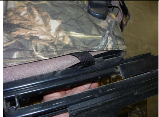
Step 10. Driver & Passenger Bottoms/DB&PB: Route the inside Velcro™ over the seat slide.
