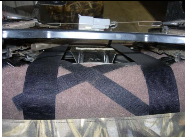
Step 15. Driver & Passenger Bottoms/DB&PB: Line up the front seam of the covers as in Step 2, then pull and fasten the Velcro™ to the seat carpet.
