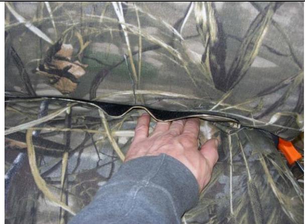
Step 16. Driver & Passenger Bottoms/DB&PB: Tuck the back edge the cover thru, then like the seat tops, use one hand in a smoothing action while pulling on the back edge of the seat cover, tightening it and pulling it back into position, again line up the seams.
