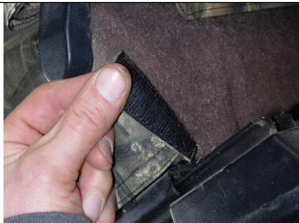
Step 17. Driver & Passenger Bottoms/DB&PB: Pull the inside edge back around and press it to the carpet on the back edge of the seat.
