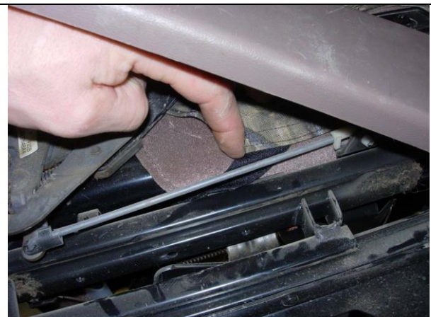
Step 12. Driver & Passenger Bottoms/DB&PB: Remove the two screws on side of the plastic cowl on the outside of the seat bottom. Route the Velcro™ where shown, behind the metal rod for the slide.
