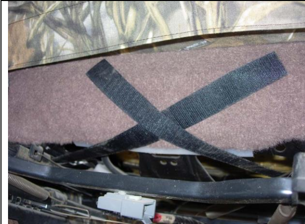
Step 13. Driver & Passenger Bottoms/DB&PB: Connect the outside edge Velcro™ at an angle to the rear edge of the seat, crossing the inside Velcro™ forming an "X".
