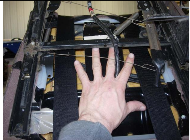
Step 14. Driver & Passenger Bottoms/DB&PB: Carefully route the long under the knee Velcro™ avoiding the seat mechanisms.
