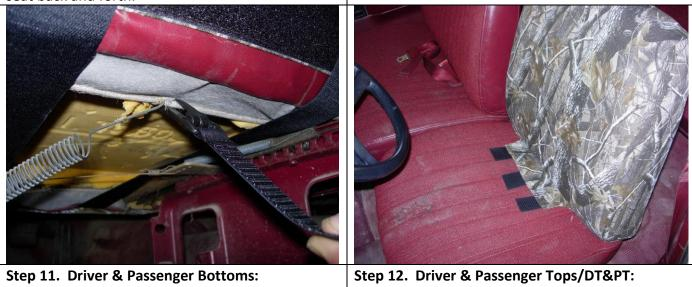
Step 11. Driver & Passenger Bottoms: View from under the driver's seat in back. Clip the 1" snap hook over the metal edge where shown under the back edge of the seat and press the Velcro<sup>™</sup> to the loop Velcro<sup>™</sup> in back. Trim the excess. Use two buckles equally spaced for the passenger side.
