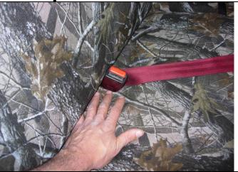
**Step 2. Passenger Bottom/PB:** Feed the seat belts through the provided opening. The seams of the seat cover should closely match the seams of your seat.
