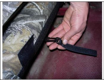
**Step 10. Driver & Passenger Bottoms/DB&PB:** View from behind the driver's seat. The 1" snap hook clips on to the back edge of the seat with the hook up.
