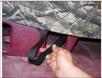
**Step 9. Driver & Passenger Bottoms/DB&PB:** View from the driver's side. Put the long outside hook Velcro<sup>™</sup> through the square opening in the seat frame and press it to the loop Velcro<sup>™</sup> in back at an angle. This Velcro<sup>™</sup> can be eliminated and cut off if it interferes too much with moving the seat back and forth.
