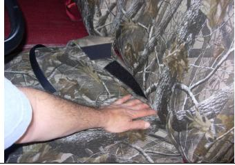
**Step 1. Driver & Passenger Bottoms/DB&PB:** Place the seat cover on with the long hook Velcro<sup>™</sup> to the front. Tuck in the back edge of the seat cover into the seat.
