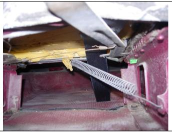
**Step 6. Driver & Passenger Bottoms/DB&PB:** View from under the driver's seat. Route the long outside edge hook Velcro<sup>™</sup> next to the seat between the adjustment lever and the tension spring as shown. Press it to the loop Velcro<sup>™</sup> on the back edge.
