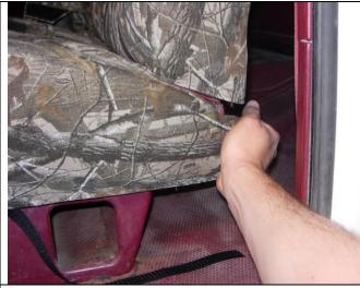
**Step 5. Driver & Passenger Bottoms/DB&PB:** View from the driver's side. Pull the outside flap around to the back and press the hook Velcro<sup>™</sup> to the loop Velcro<sup>™</sup> the same way as step 4.
