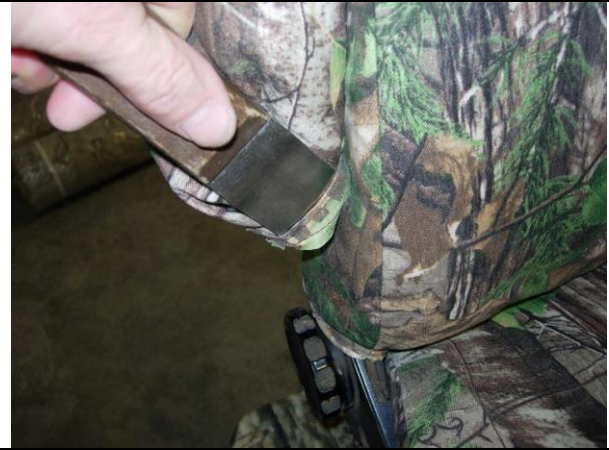
Step 22. Driver and Passenger Armrests Using a similar tool shown such as a shoe horn, use the tool to force the cover over the front corner.
