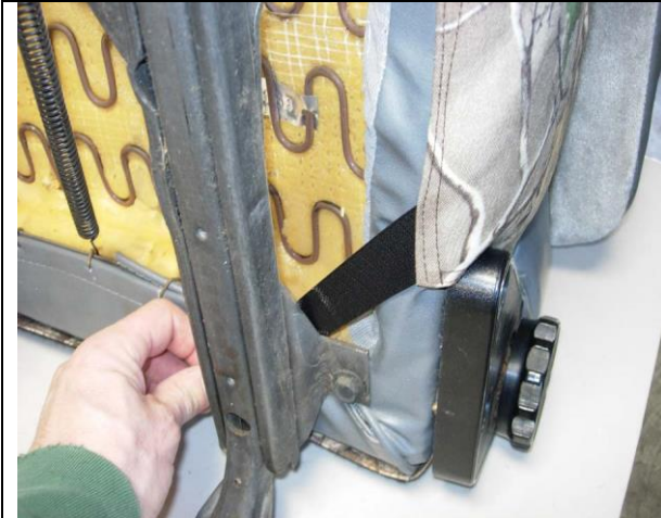
Step 5. Driver and Passenger Bottoms/DB&PB: Route the side Velcro™ over the top of the seat slide at an angle to the back edge.
