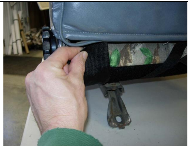
Step 8. Driver and Passenger Bottoms/DB&PB: Connect the hook Velcro™ to the loop Velcro™ on the back edge. Do this by pulling on the back of the seat cover while using one hand in a smoothing action from front to back pulling the seat cover tight, then connect the Velcro™.
