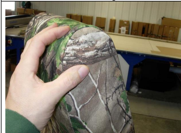
Step 13. Driver and Passenger Tops/DT&PT: Pull the cover down and form it to the top of the seat.
