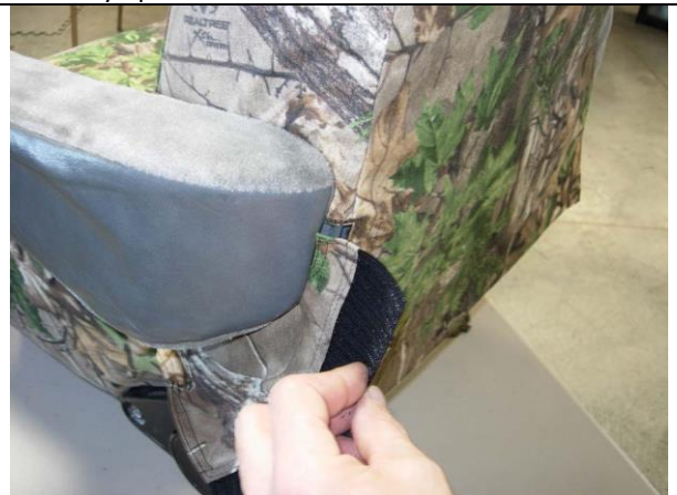
Step 14. Driver and Passenger Tops/DT&PT: Tuck the seat cover under and behind the armrest.
