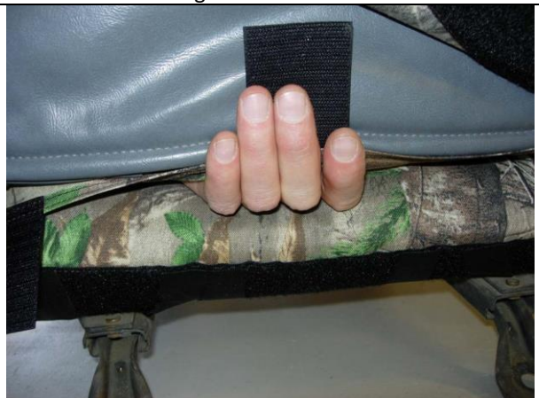
Step 18. Driver and Passenger Tops/DT&PT: Same as Step 8, use one hand in a smoothing action down the front of the seat cover from top to bottom while gently pulling on the Velcro™ from behind, press it to the seat with the front hand, then press it to the loop Velcro™ sewn inside the back edge.
