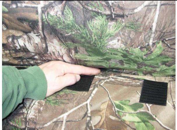
Step 16. Driver and Passenger Tops/DT&PT: Tuck in the front edge Velcro™.
