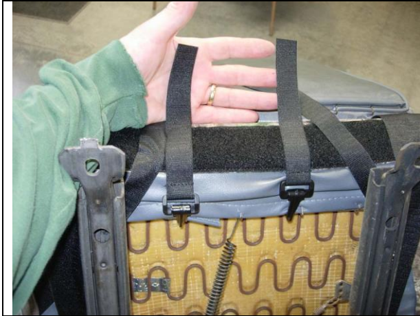
Step 9. Driver and Passenger Bottoms/DB&PB: Connect the two plastic hooks with Velcro™ sewn to them where shown, then press them onto the loop Velcro™.
