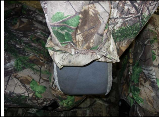
Step 21. Driver and Passenger Armrests Make sure the back of the cover is turned inside out.
