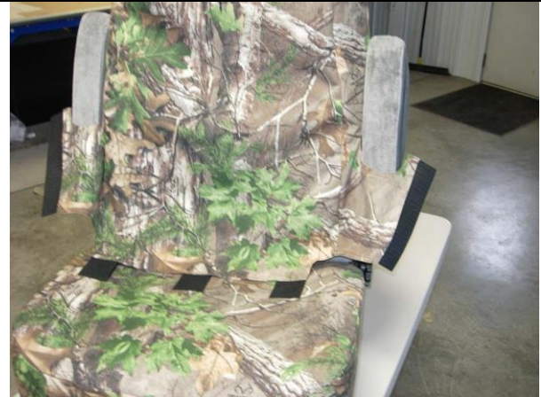
Step 12. Driver and Passenger Tops/DT&PT: Carefully open the seat cover bottom and sides.
