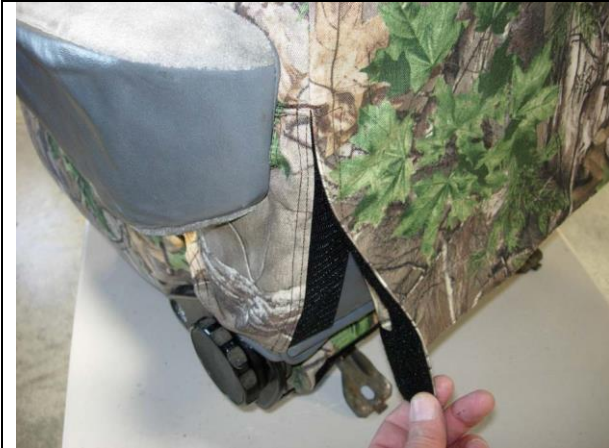
Step 15. Driver and Passenger Tops/DT&PT: Connect the vertical Velcro™.
