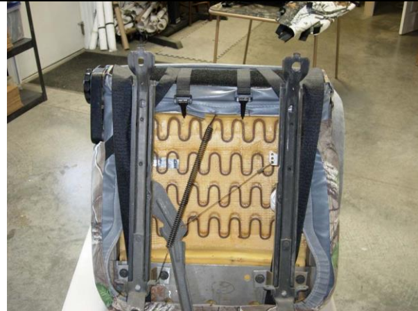
Step 11. Driver and Passenger Bottoms/DB&PB: View from under the seat showing the Velcro™.
