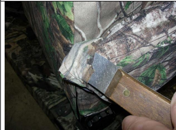
Step 23. Driver and Passenger Armrests Use the tool to pry the cover over the top side of the armrest. This will be very tough to do, as the cover is so tight.
