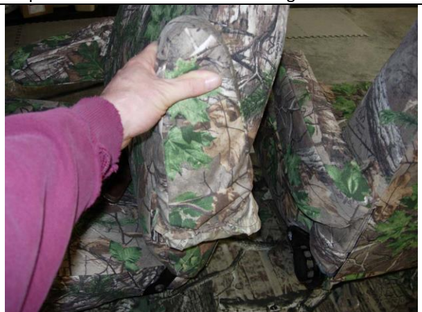
Step 20. Driver and Passenger Armrests Form the cover to the front of the armrest making sure it's pulled down all the way.
