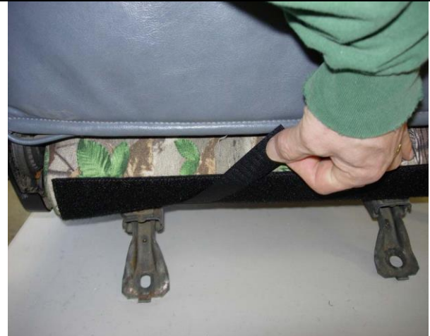
Step 6. Driver and Passenger Bottoms/DB&PB: Press the hook Velcro™ to the loop Velcro™ on the back edge.
