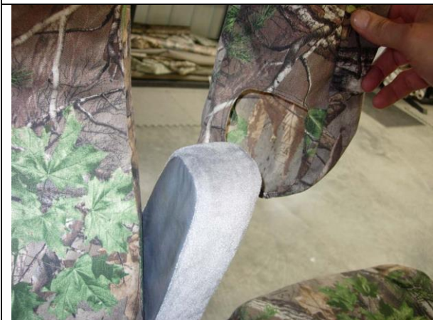
Step 19. Driver and Passenger Armrests/DAL, DAR, PAL, PAR: Slide the covers on with the opening to the inside.
