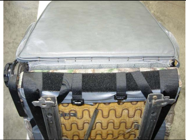
Step 10. Driver and Passenger Bottoms/DB&PB: Trim the excess Velcro™. Finished, the Velcro™ should look like this.
