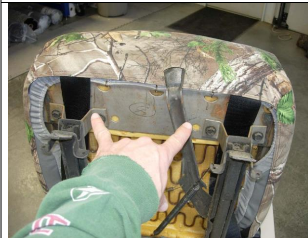
Step 7. Driver and Passenger Bottoms/DB&PB: Route the two long hook Velcro™ under the seat where shown.
