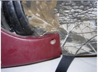
Step 4. Bottom: Tuck the sides of the seat cover between the plastic and the seat on both sides as shown.
