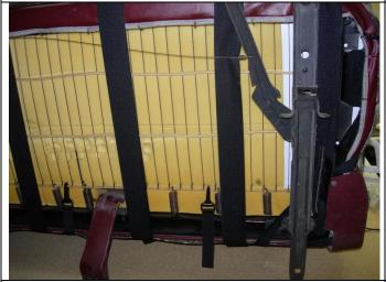
Step 3. Bottom: Position the seat cover by lining up the seams of the seat cover to the seams of the seat. Pull on the back edge of the seat cover with one hand and use your other hand in a smoothing action from front to back, then route the front hook Velcro<sup>™</sup> under the seat and connect them to the loop Velcro<sup>™</sup> sewn on the back edge. Be sure to route the Velcro<sup>™</sup> avoiding the seat slide wire.
