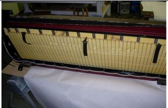
Step 6. Bottom: Clip the three plastic clips with Velcro<sup>™</sup> sewn to them onto the metal bar under the back edge where shown.
