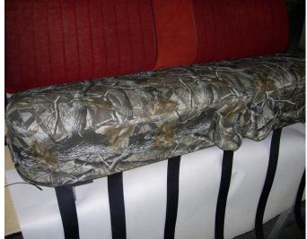
Step 2. Bottom: Place the seat cover on with the long hook (sticky) Velcro<sup>™</sup> to the front and feed the seat belts through the provided openings.
