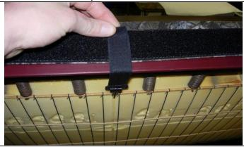
Step 7. Bottom: Connect them to the loop Velcro™ sewn on the back edge. Trim excess.
