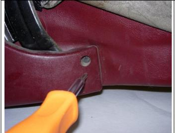
Step 1. Bottom: Temporarily remove this Phillips screw from both sides.
