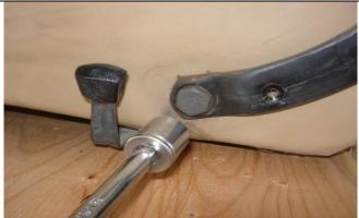
Step 2. Bottom: Temporarily remove the bolts on the left and right using a socket or end wrench.
