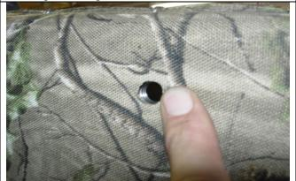
Step 5. Bottom: After the seat cover is centered left and right, feel for the hole for the side bolts and trim it out with a scissors. The hole can be larger than shown because of the large washer.
