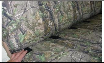
Step 10. Top: Slide the seat cover top on with the extending hook Velcro™ to the front and tuck them into the seat.
