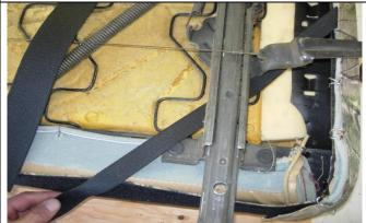
Step 6. Bottom: Route the long side hook Velcro™ at an angle, over the seat slide, and then press it to the loop Velcro™ sewn on the back edge.
