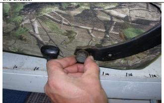
Step 9. Bottom: Re-attach the backrest to the seat bottom. Put the side plastic pieces back on.
