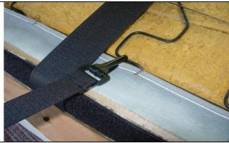
Step 8. Bottom: Fasten the no slip buckle under the back edge of the seat and connect the hook  $Velcro^{TM}$  to the loop  $Velcro^{TM}$ .
