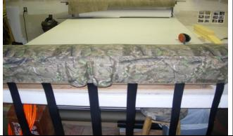
Step 3. Bottom: Place the seat cover on with the long hook (sticky) Velcro<sup>™</sup> to the front. Route them under the seat and connect them to the loop Velcro<sup>™</sup> sewn on the back edge, avoiding the seat mechanisms.
