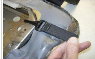
Step 7. Bottom: Connect the side plastic buckles to framework under the seat, then connect it as shown, trim the excess.
