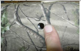
Step 5. Bottom: After the seat cover is centered left and right, feel for the hole for the side bolts and trim it out with a scissors. The hole can be larger than shown because of the large washer.
