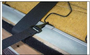
Step 8. Bottom: Fasten the no slip buckle under the back edge of the seat and connect the hook Velcro<sup>™</sup> to the loop Velcro<sup>™</sup>.
