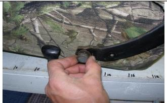
Step 9. Bottom: Re-attach the backrest to the seat bottom. Put the side plastic pieces back on.
