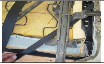
Step 6. Bottom: Route the long side hook Velcro<sup>™</sup> at an angle, over the seat slide, and then press it to the loop Velcro<sup>™</sup> sewn on the back edge.
