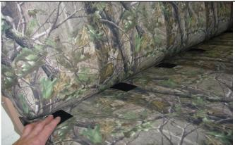
Step 10. Top: Slide the seat cover top on with the extending hook Velcro<sup>™</sup> to the front and tuck them into the seat.
