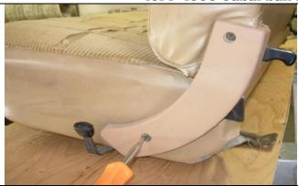
Step 1. Bottom: Temporarily remove the two screws on the plastic side panel on both sides using a Phillips screwdriver.
