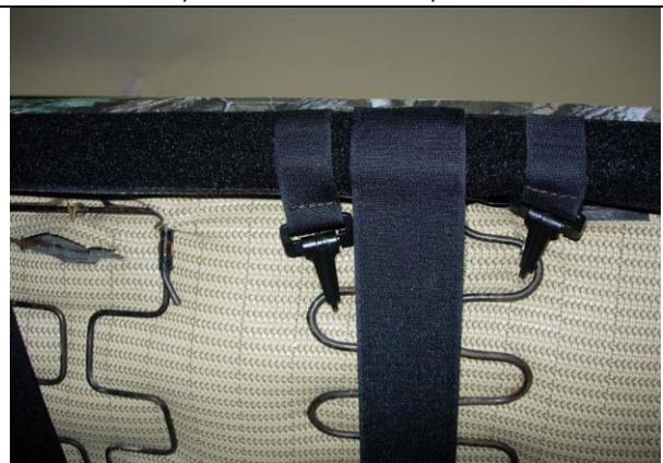
Step 10. Bottom/B: Connect them under the seat where the driver & passenger will be sitting, then press them to the loop Velcro™.
