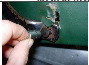
**Step 1. Prepare the seat for installation:**Using an Allen Wrench or proper sized socket stud, remove the backrest from the set bottom.
