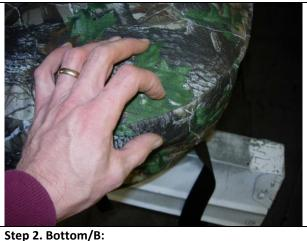
All the parts of the seat cover are labeled on the inside right front corner. Use the "Seat Cover Part ID Chart" to ID parts. Place the bottom on with the long hook (sticky) Velcro™ to the front. Pull the cover around the back corners, then pull it over the front. Work the material inside the seat cover outward, from forefinger to thumb as shown.
