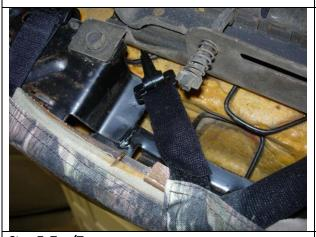
Step 7. Top/T: View from under the side of the seat. Notice the two Velcro™ sewn on each side with the plastic buckle. Connect the front Velcro™ buckle as shown.
