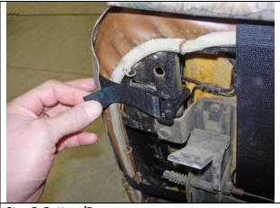
**Step 5. Bottom/B:**Disconnect the Velcro™ to gain grabbing length.
