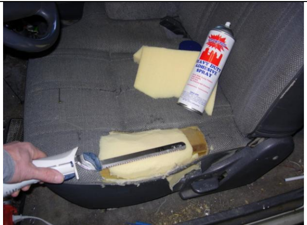
Use 3M 08080 spray glue to glue the repair foam to the seat. Use the electric knife to shape it to the seat.
