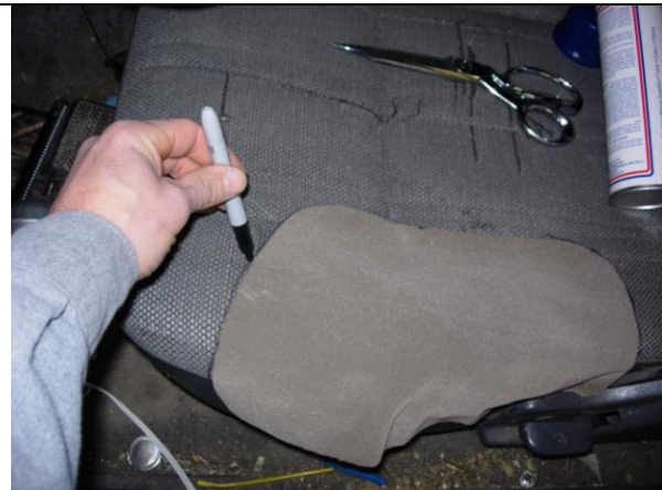
Cut the cloth making it at least 2" larger than the cut-out. Dry fit the piece and mark the border with a pen, and then glue it to the seat.
